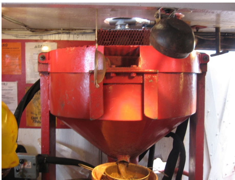
Figure 16: Rotary Splitter at work
