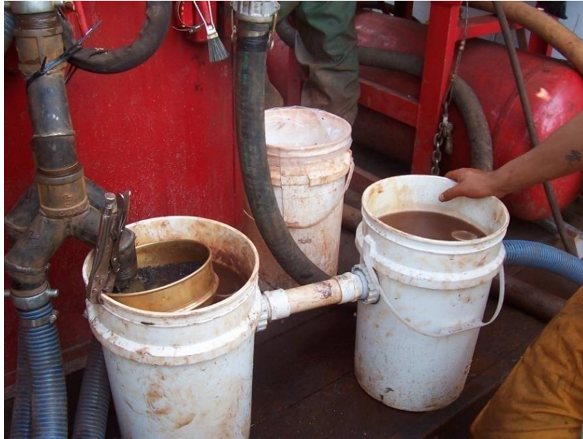
Figure 14: RC Size Reduction and Sampling Setup
