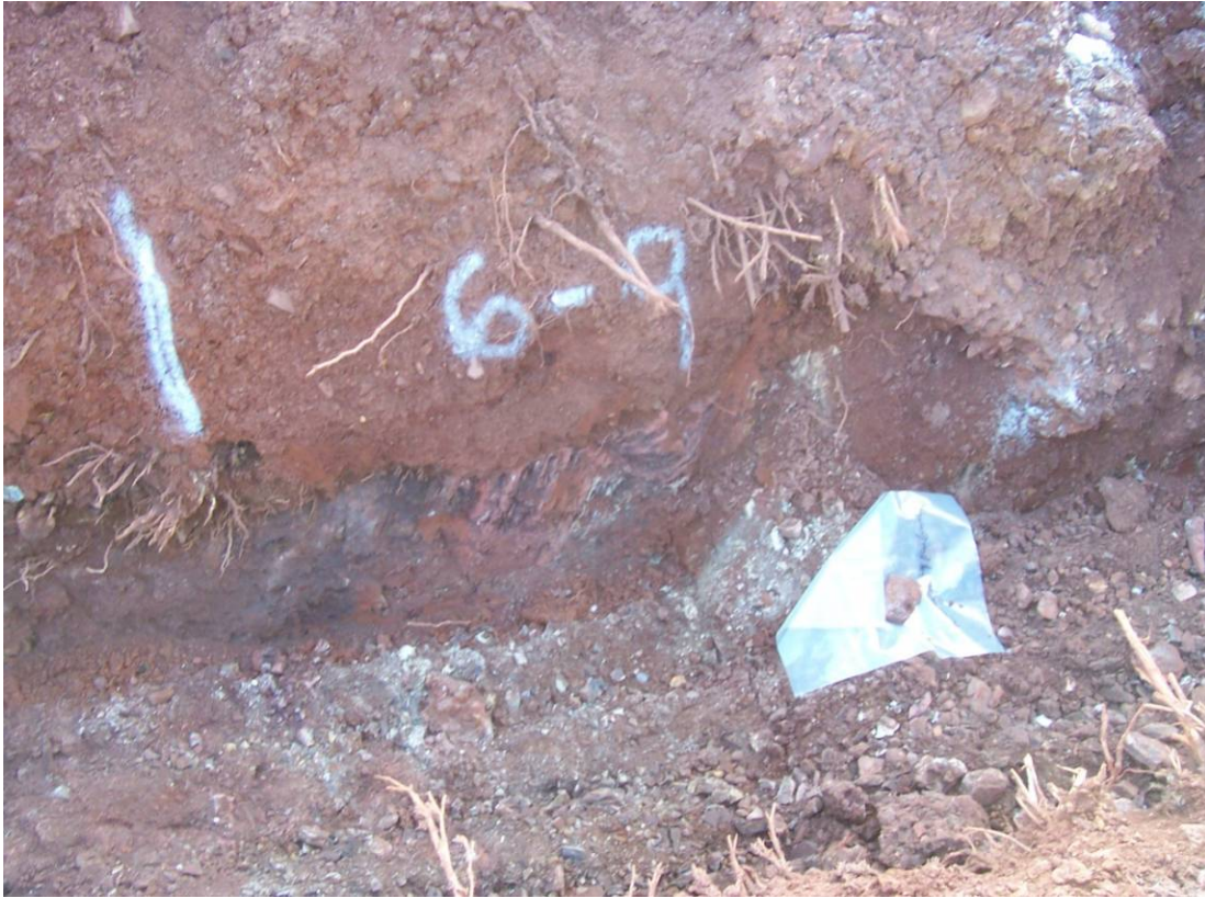
Figure 17: Trench sampling intervals
