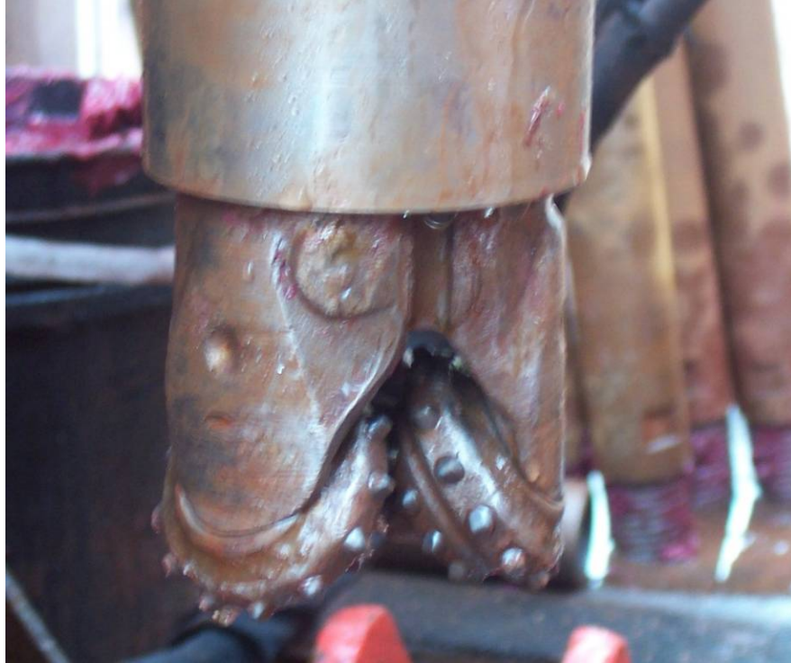
Figure 11: RC Tricone Bit
