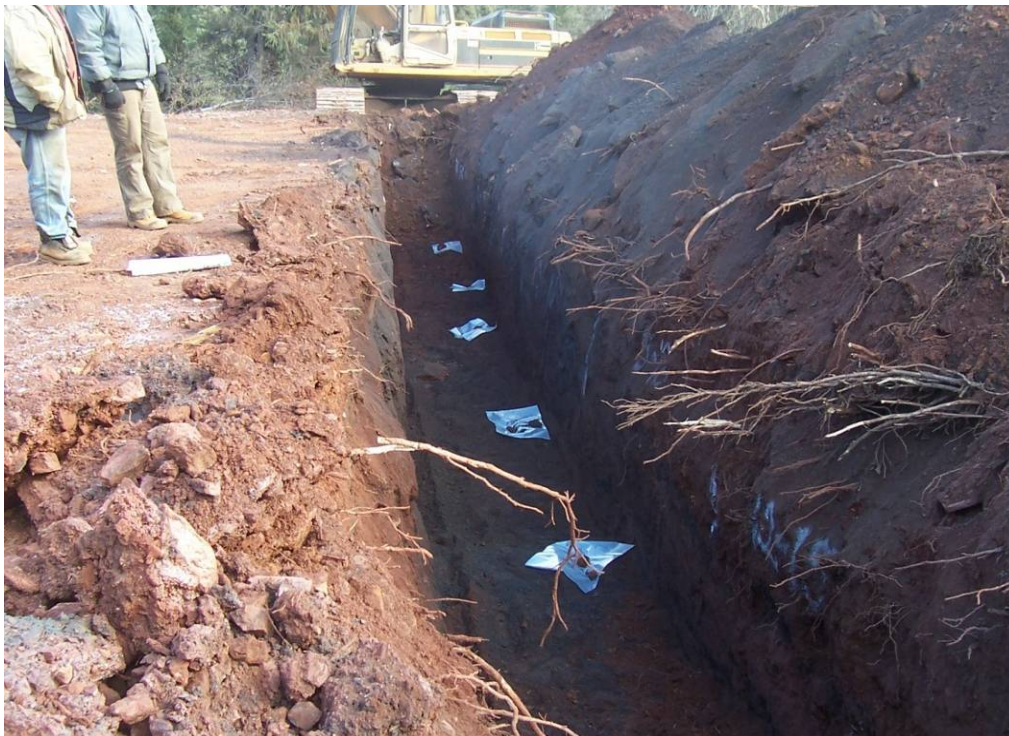
Figure 19: Trench sample layout at James
