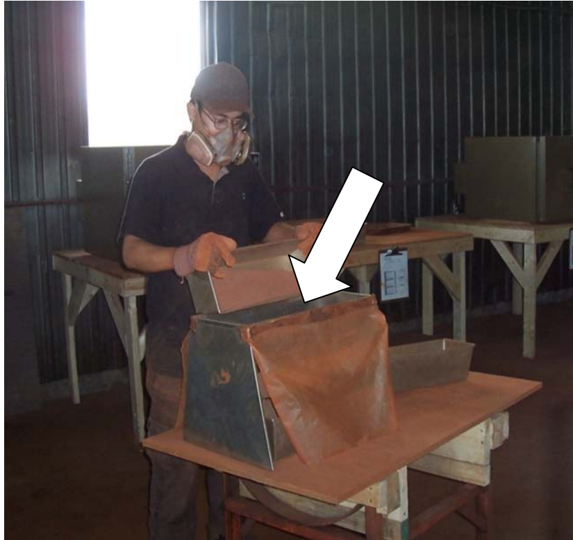
Figure 21: Sample Size Reduction with a Riffle Splitter
